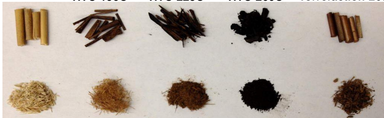
Raw HTC-190C HTC-225C HTC-260C Torrefaction-260C
