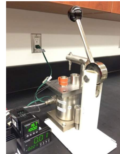
Pelletization Pressure: ~ 9 MPa Temperature: 100°C
