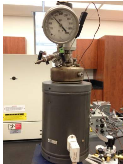
Hydrothermal reactor Pressure: ~ (1.2-5 MPa) Temperature: 190-260°C
