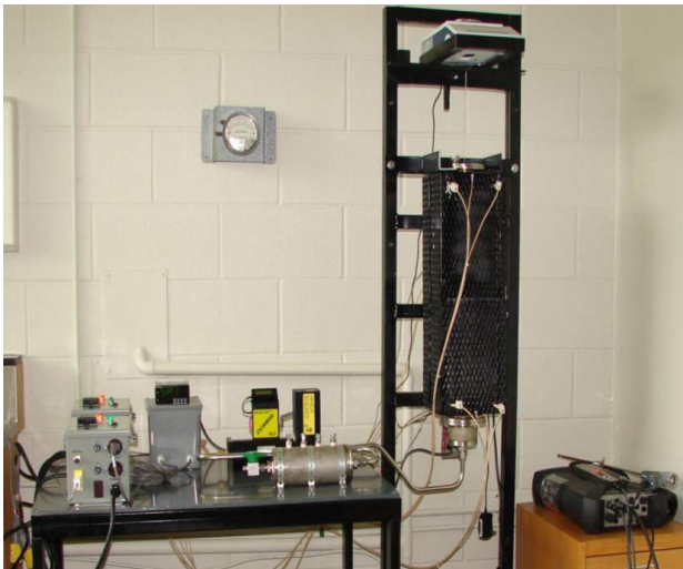
Custom build Macro TGA (a tubular reactor for slow pyrolysis (200-800 C))
