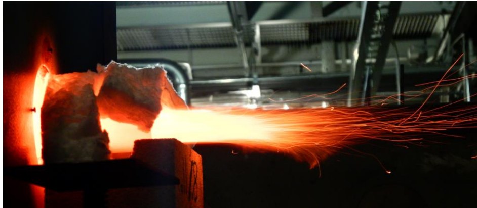
Pulverized coal injection simulation rig
