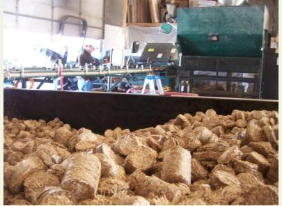
Bales are busted---- (density 2-3 lb/ft<sup>3</sup>) Switchgrass is compacted into briquettes--- (density 30-35 lb/ft<sup>3</sup>) Briquetting reduces the storage volume & improve handling Need to achieve 2 ton/hr
