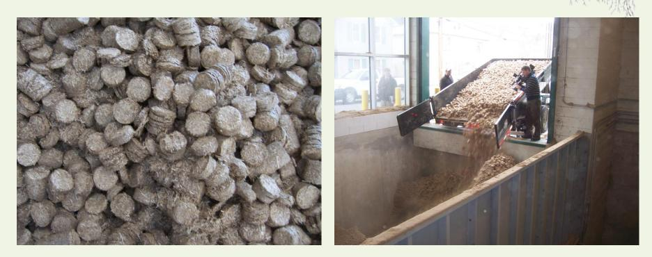
Briquettes are dumped into storage pit Augers transport to fuel to the boiler Briquettes are easier to handle than loose chopped
